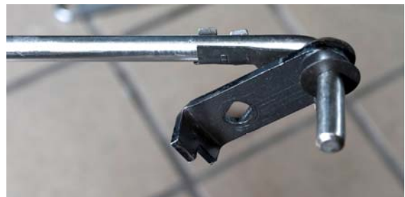
Figure 5 The rear valve switch is shown in place. It is wired in parallel with the existing switch, using piggyback terminals.
